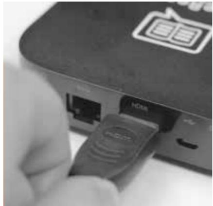
2. Connect the other end of the HDMI cable into an available HDMI port in the back of your TV
