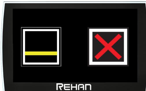
Tap the cross box to re-enable the horizontal reading line.
